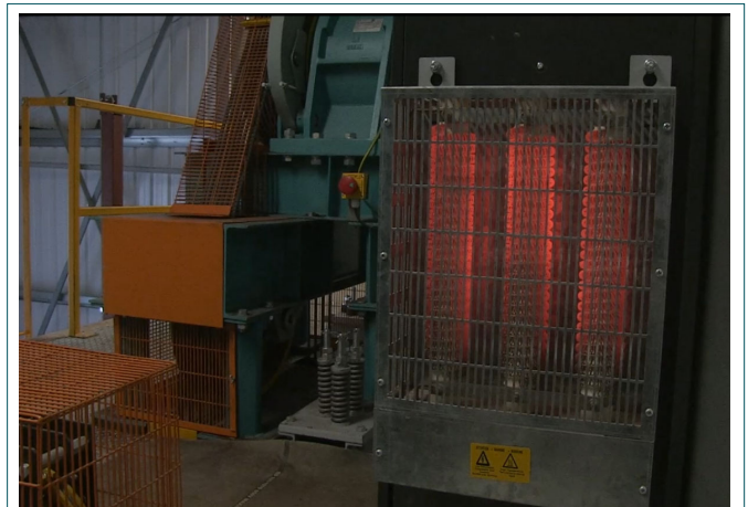
Before: Excess Energy Lost Through Braking Resistors
