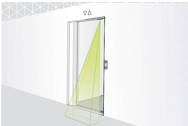
IMS 100 NT - corner-mounted for side-opening doors
