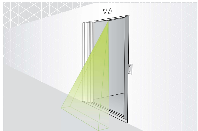
IMS 100 NT - center-mounted for center-opening doors
